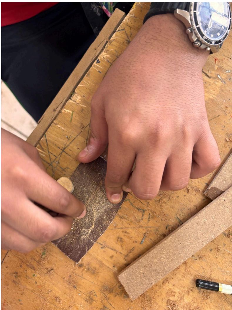
Sanding, here you can see me sanding the wood after it was cut
